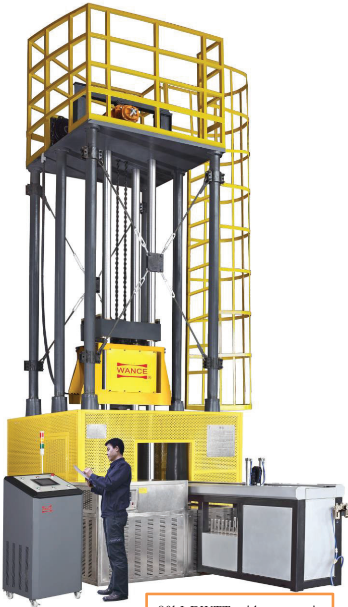
80kJ DWTT with automatic feeding and cooling
