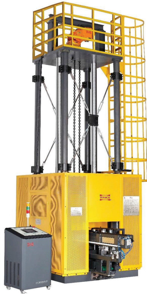
50kJ DWTT with semi-automatic feeding and cooling
